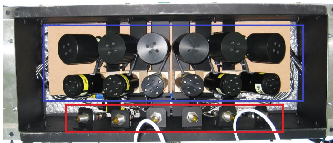
Figure 3-5. Optical sensor box with 12 multi-spectral radiometers (two upper rows indicated by blue box) and 6 thermal infrared radiometers (bottom row indicated by red box)
