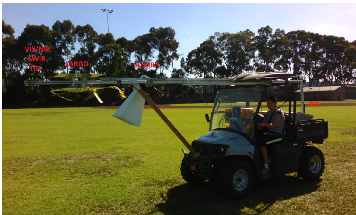
Figure 6-9. Buggy platform, consisting of ELBARA III, multi-spectral sensors (VNIR, SWIR, and TIR), GNSS-R sensor (LARGO), and EM38.
