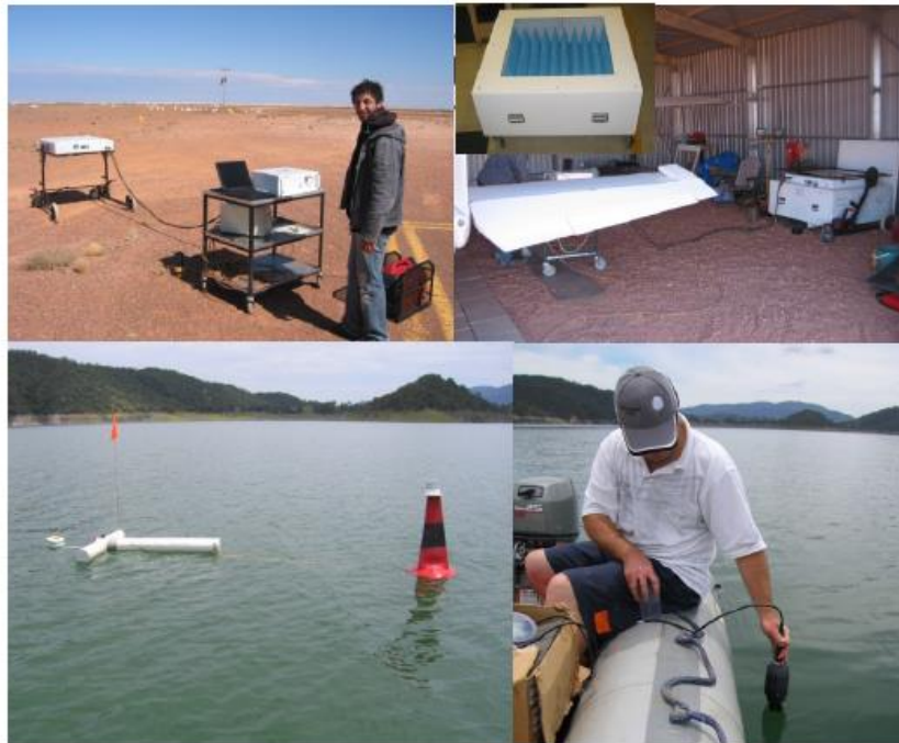
Figure 5-7. Upper left: undertaking a sky cold point calibration with PLMR; upper right: undertaking a warm point calibration with the calibration box shown in the inset; lower left: the buoy used to monitor water temperature and salinity; lower right: undertaking a boat transect of water salinity and temperature.
